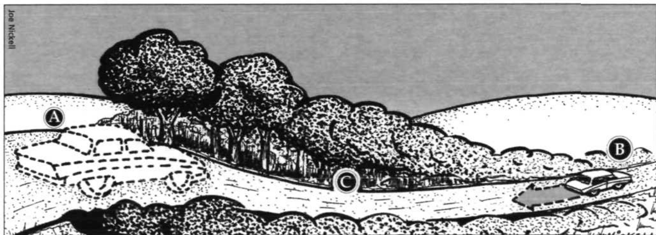
Figure 2. Magnetic Hill. Driver proceeds from point A along an apparently continuous downhill course to B, places vehicle in neutral and removes foot from brake pedal. Vehicle seems mysteriously drawn backward, but in fact the distance from B to C is a slightly downward incline and momentum propels the vehicle back to A.
